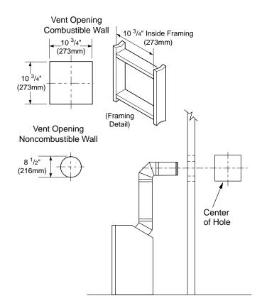
Figure 9 - Vent Opening Requirements
